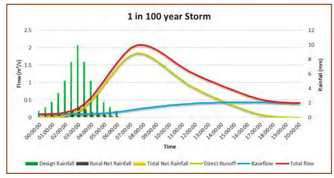
Figure 7: Design Hyetograph and Hydrograph for the natural catchment using FEH Catchment Descriptors
