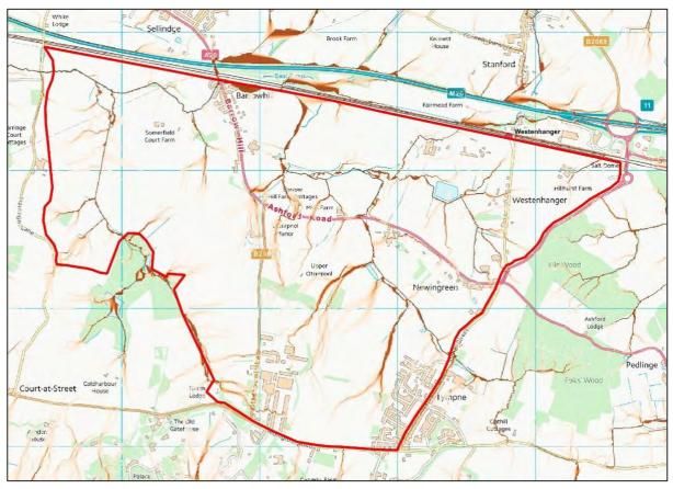
Figure 3: Flow accumulation from LiDAR/OS DTM (darker orange equates to more accumulation)
