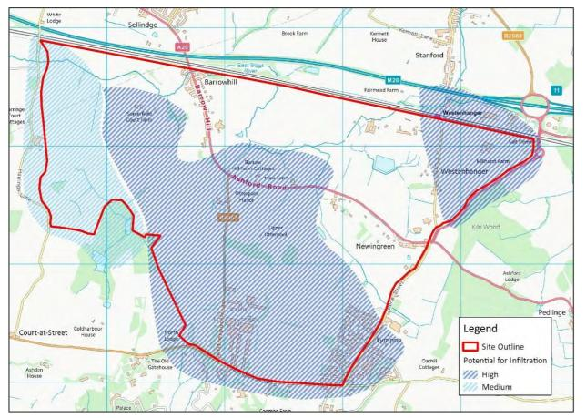
Figure 11: Potential for Infiltration Map (Source: Arcadis. Contained OS Opendata)
