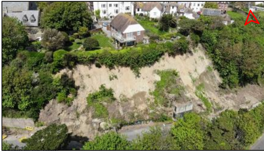
Photo 5 - Aerial image showing the extent of the landslide / slip at S3 along the eastern section of the Road of Remembrance.
