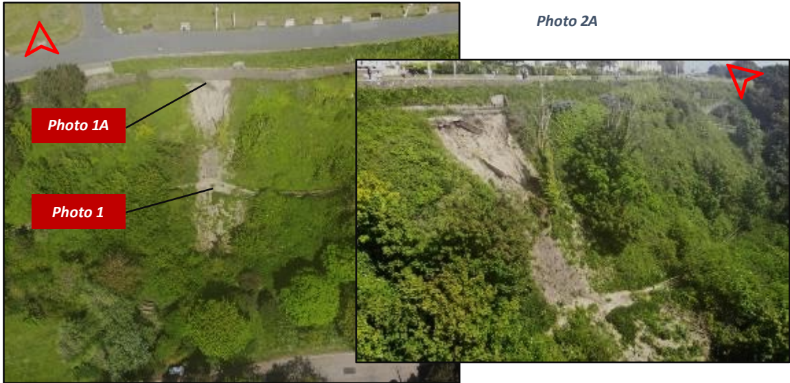
Photo 2/2A - Aerial images showing the extent of the landslide / slip from the footpath below the promenade across the intermediate footpath between the promenade and the coastal path and further south between the intermediate footpath and the coastal park.
